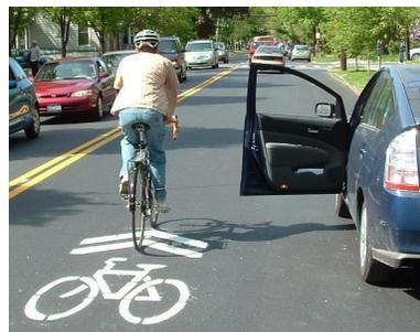
**Figure 5:** Photo of sharrow marking on Cayuga St. The image shows the correct positioning of a cyclist passing a parked car.
