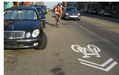
**Figure 3:** Current design of sharrows - example from Pittsburgh.
